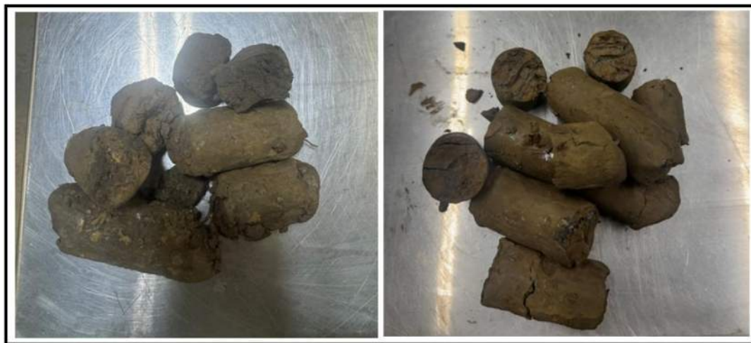
Figure 3: Stratum II Materials Left: S2B1 / S-1 (CL Materials) Right: S2B4 / S-6 (CH Materials)
